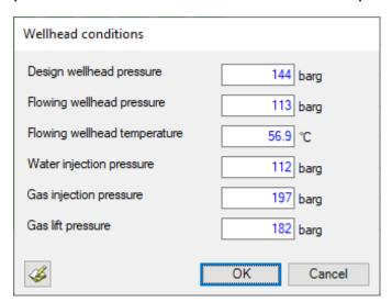
Water injection, gas injection and gas lift pressure are only relevant if these services are selected. Adjust the conditions as necessary and then click **OK** to move onto the Concept selector form.
