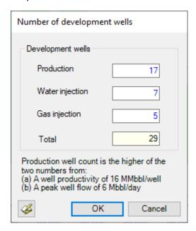
The default number of production wells is based on the recoverable reserves, well productivity, plateau production and peak well flow. The default number of water injection wells assumes an average of two injectors for every five oil production wells. Gas injectors are based on an average flowrate of 30 MMscf/day per well.
