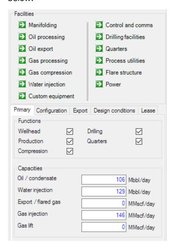
The input form shows the main design parameters for a given component, such as the design flowrates. You can make changes to these values to match your design assumptions. When you click **Apply** these changes will be applied to the component and the CAPEX estimate adjusted accordingly.
