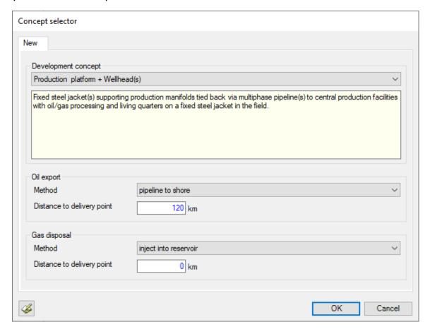
QUE\$TOR selects a field development concept based on the field level data and production profile. You can change this to another of the 14 default concepts using the list box. If you want to configure your concept from scratch, select 'Blank concept'.
