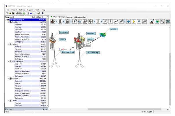
The field development schematic shows the components within your chosen concept on the right hand side of the screen, with the associated high level CAPEX summary on the left hand side of the screen.
