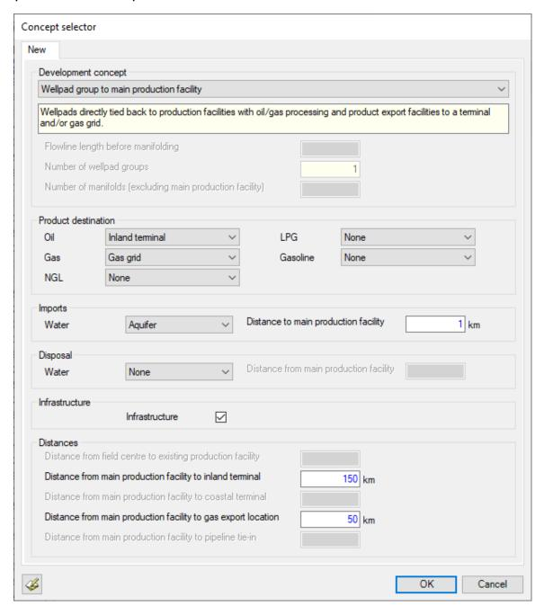
QUE\$TOR selects a field development concept based on the field level data and production profile. You can change this to another of the 6 default concepts using the list box. If you want to configure your concept from scratch, select 'Blank concept'.
