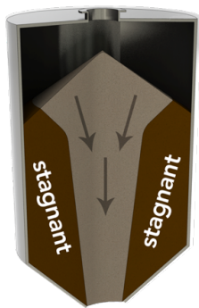
Surge bin discharged in "Funnel Flow"
