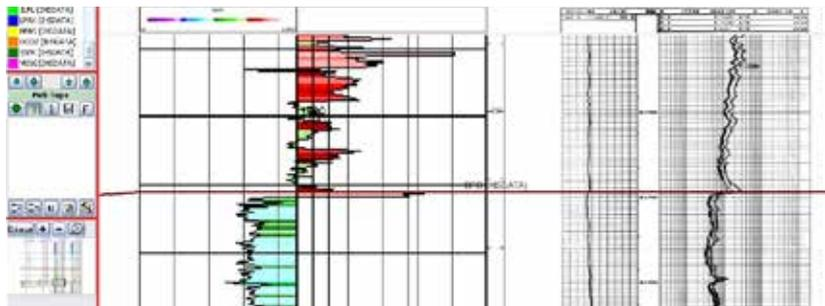
Quickly pick tops on digital and raster logs using the Log Correlation Module, and interpolate between wells based on log data using the interpretive color fill functionality.
